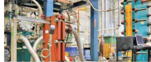
Heat exchanger development & testing lab
