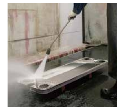
Water jet cleaning
