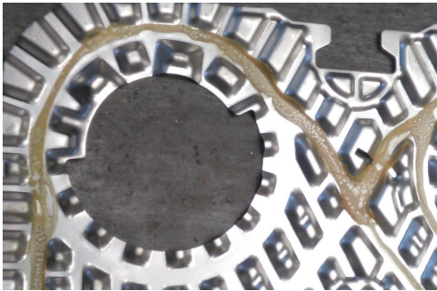
Photo 1. Plate on which adhesive remains
