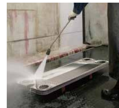
Water jet cleaning
