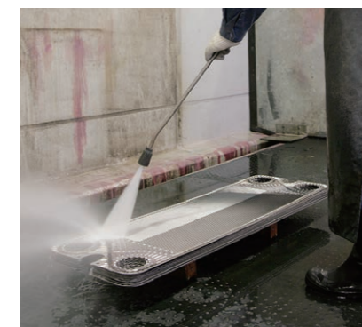
Water jet cleaning
