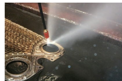
Hot Water Jet Cleaning
